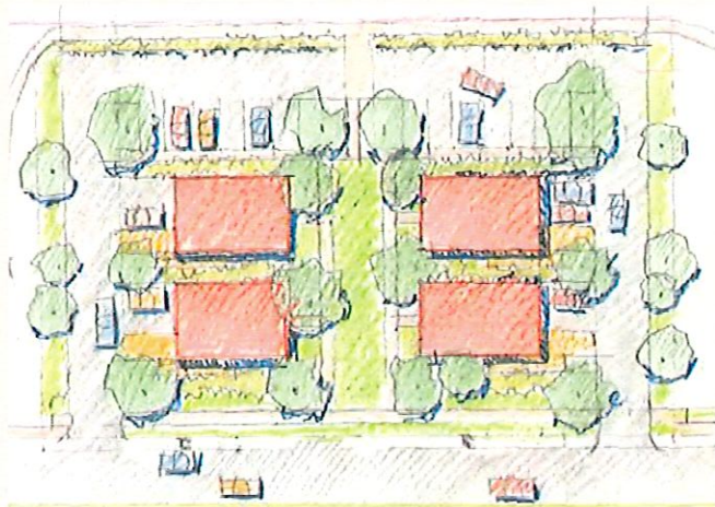
An alternative layout includes residences that front on a shared greenspace and distributed parking with canopy trees.
